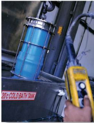
Hydrostatic Pressure Test
